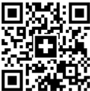
Technically speaking, overlaying images over QR codes is possible because QR codes implement *error correction*, which means that a QR code can still be read by a scanner even though part of it is damaged or covered by an image. The QR code specification lists the following error correction levels and their corresponding theoretical recovery rates (the percent of the coding words that can be missing without affecting the QR code's readability).
