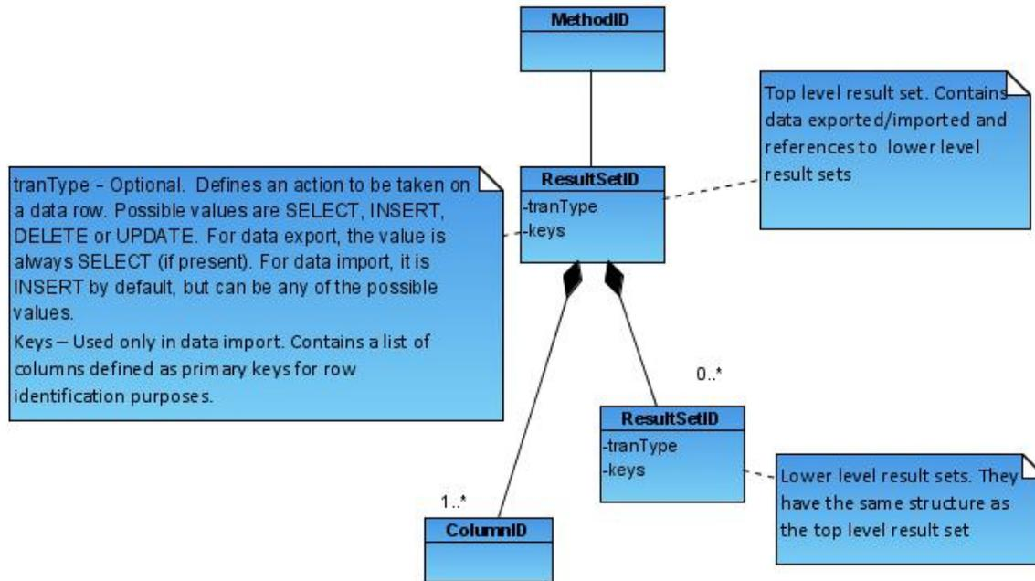
Because the Data Integration application supports result set trees that can contain many levels, data is arranged in the “Russian Doll” format, in which child rows belong to their parent row. The opposite would be the “Flat” format, in which all result set rows are on the same level.
