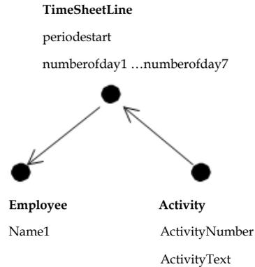
In the second query, the first selected field is EmployeeNumber from the object Employee. The least spanning tree does not contain the Activity object, indicating that the object is not needed in the generated SQL query.
