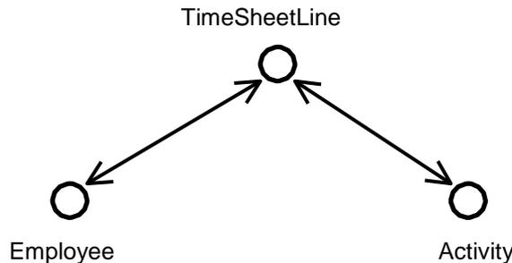
A query selects fields from the objects used in the universe, thereby selecting vertexes in the graph. The first field selected in the query selects the root of the tree. Now the least spanning tree marks the objects needed in the query.
